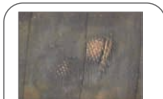
Exhaust hose with cover worn, exposing reinforcement
