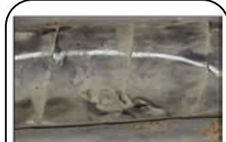
Hole in hose cover that exposes reinforcement
